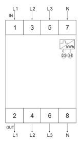
To perform a measurement, an external source + 5V DC must be connected from the pulse output to terminal 23, and the signal output to terminal 24.
